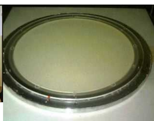
The NaI crystal of a gamma camera.
