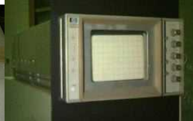
The cathode ray oscilloscope (CRO) of a gamma camera.
