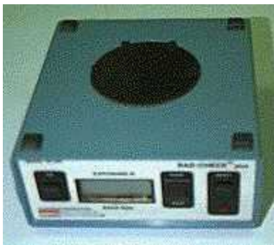
An exposure meter used in radiography.
