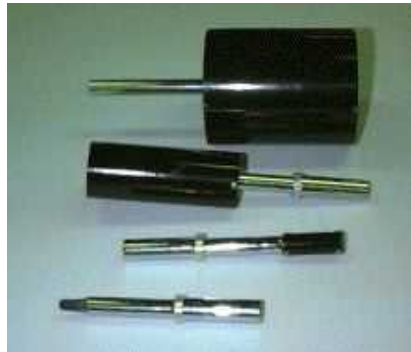
A range of ionisation chambers of different volumes using for measuring radiation exposure.
